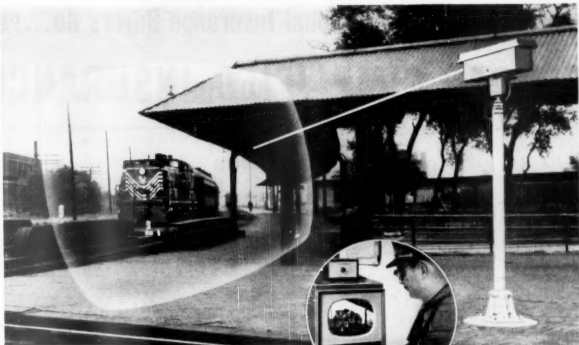
1. A weather-proof, rotating Farnsworth TV camera, mounted on the platform of the Rock Island's busy Englewood station, scans the main-line crossing.
